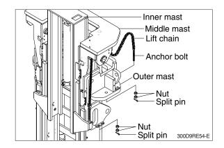
④ Pull the chains out of the sheaves and drape them over the front of the carriage.
