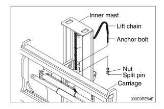
③ While supporting lift chains, remove the split pin and nuts from the anchor bolt at the lift chain side.
